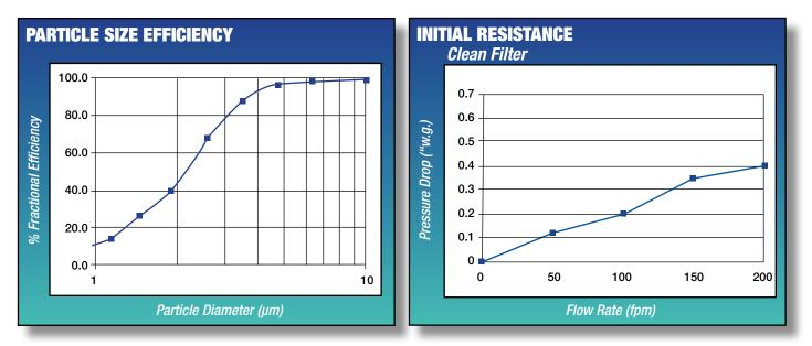
\*Filter tested per ASHRAE 52.2, Test Aerosol KCl, Neutralized. This test data is based upon clean filter performance. All filters increase in efficiency with dust loading.
